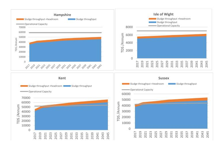
Figure 7 Projected sludge demand and capacity
