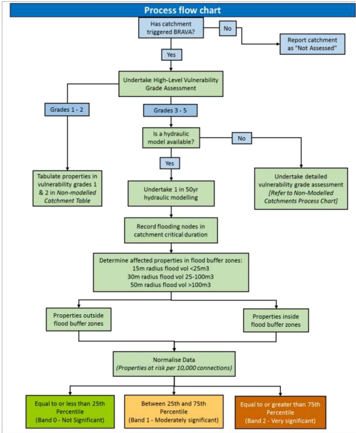
Figure 2: Process flow chart for risk of flooding due to 1 in 50 year storm (Non-Modelled Catchments)
