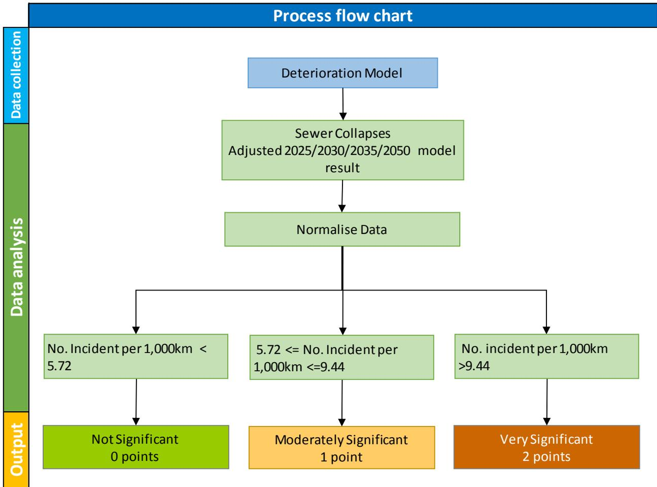
The change in predicted collapses and bursts, based on the outputs from the deterioration model, is applied to the 2020 baseline assessment for each sewer catchment to produce a predicted number of incidents per 1,000km for each future scenario.
