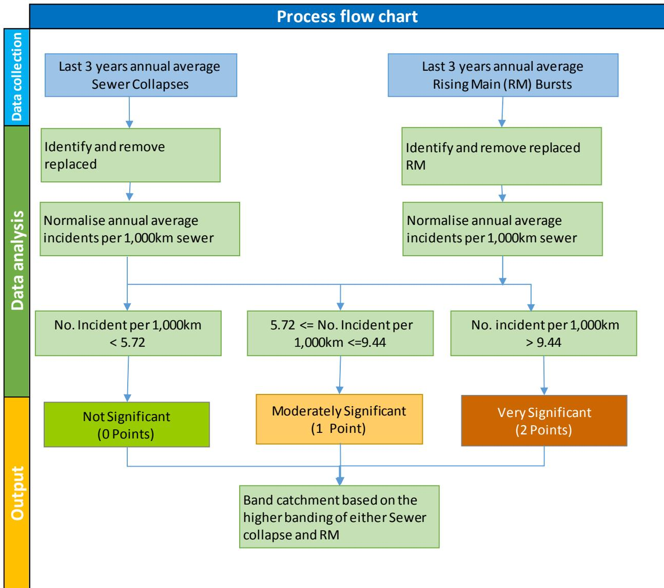
The repaired or replaced sewer and rising main data identifies assets that have been remedied after a collapse or burst incident has occurred. These incidents are removed from the number of incidents considered in the current BRAVA risk assessment as the risk has been reduced or removed due to the investment in those assets.
