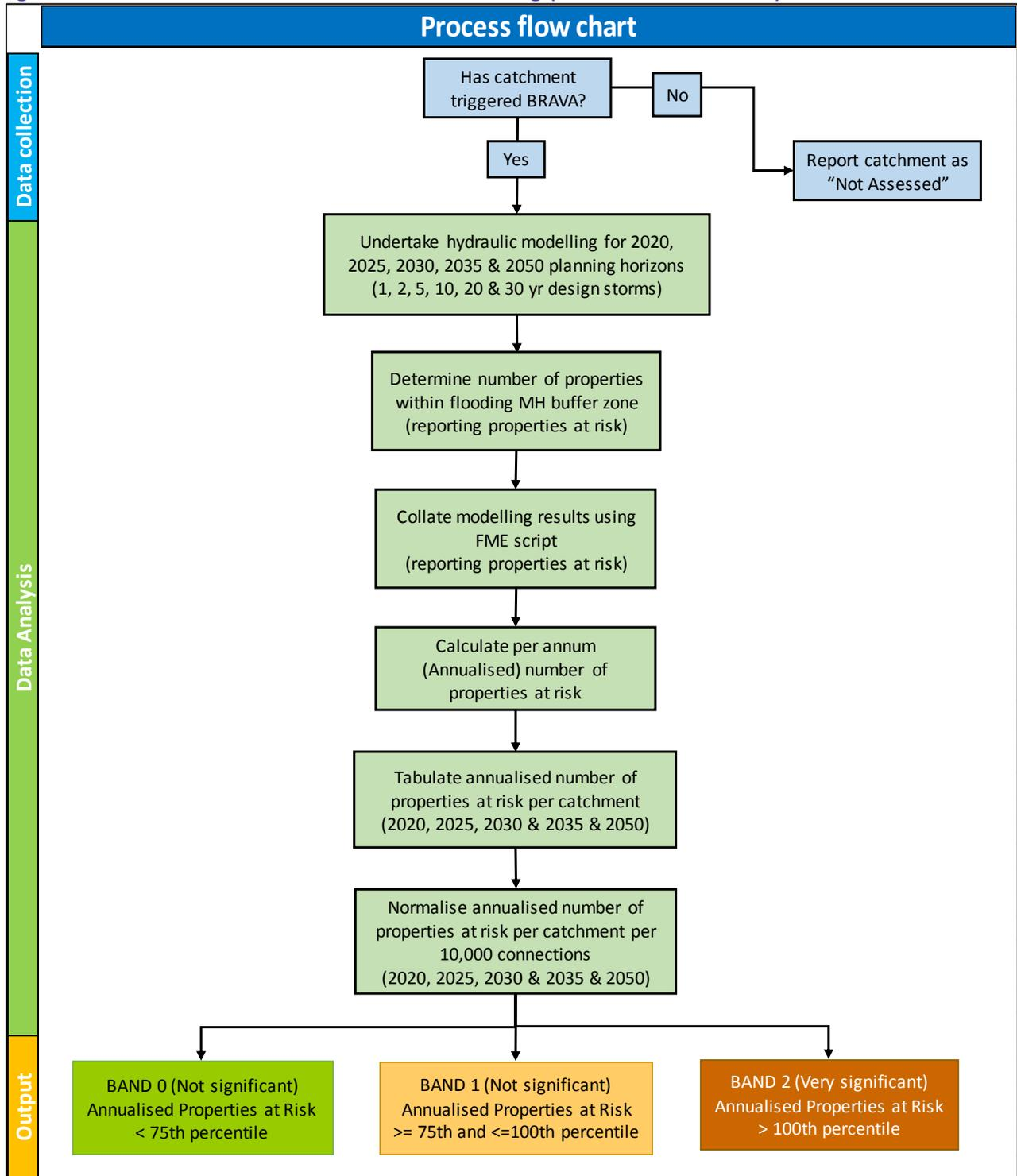
Figure 2: Process flow chart for assessing risk of flooding (Non-Modelled Catchments)
