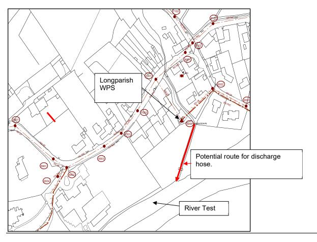
Refer Longparish IRP for further details of potential overpumping arrangement.
