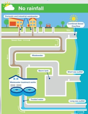
During dry weather the flow of wastewater from domestic and industrial properties is treated to meet strict bathing water standards, including UV disinfection, and then released into the sea via the long sea outfall, 2.7km offshore. Swalecliffe WTW is designed and permitted to treat 205 litres a second (I/s) of waste water.
