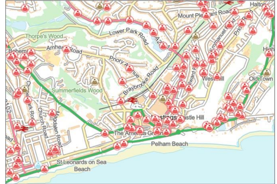
Sewer Level Monitors in the Hastings and Bexhill areas, which provide early warning of potential sewer blockages
