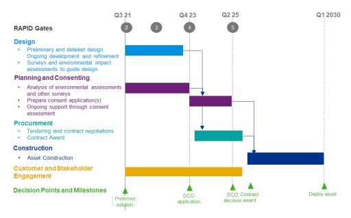
Figure 8 - High-level delivery schedule - Havant Thicket
