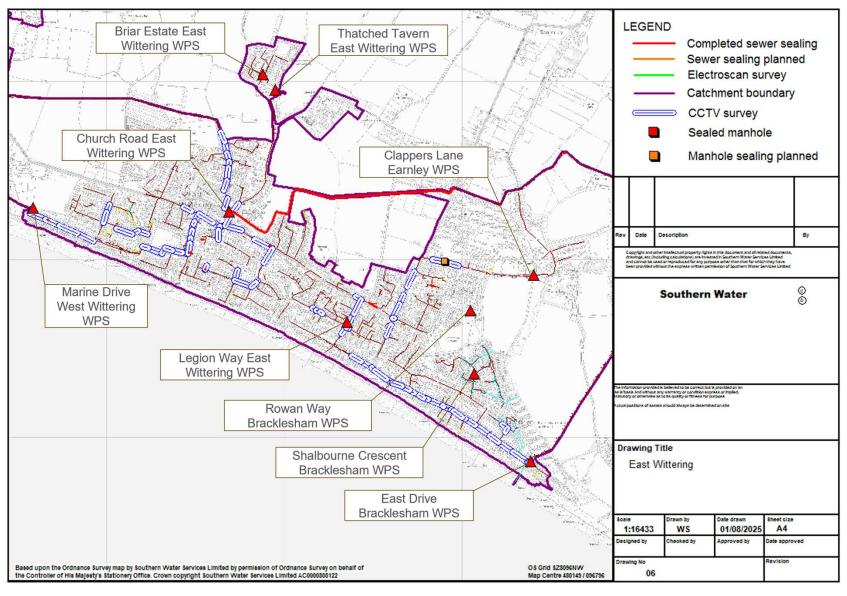
Note – sewers shown as surveyed by cctv or electro scan with no corresponding sealing work have been determined to not require rehabilitation.
