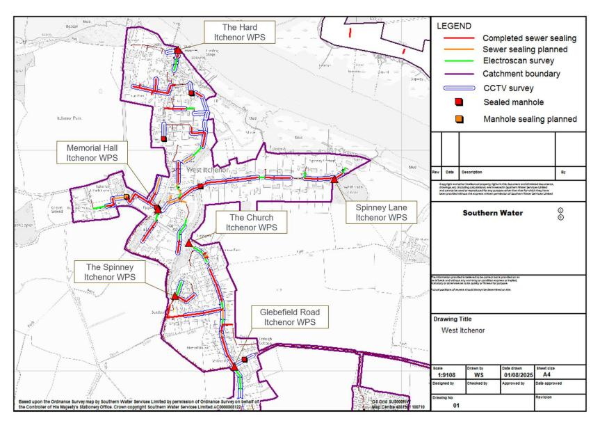
Note – sewers shown as surveyed by cctv or electro scan with no corresponding sealing work have been determined to not require rehabilitation. The use of storm harvester data will be used at some point in the future to target inspections and find infiltration
