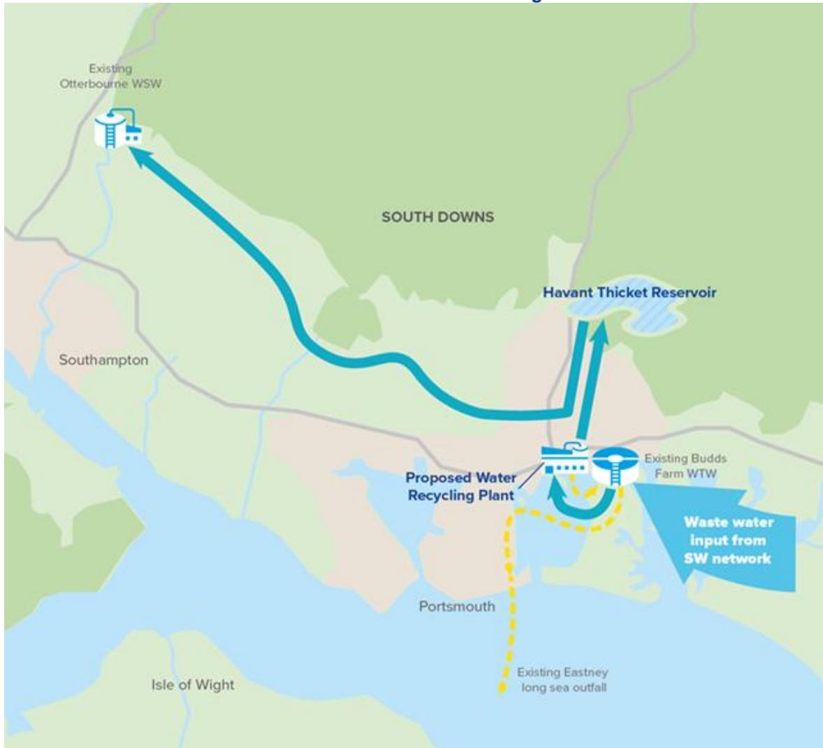
The location of the proposed scheme is at the north end of Langston harbour near Portsmouth. A waste treatment works (WTW) will supply water to a water recycling plant (WRP), which transfers recycled water to the Havant Thicket Reservoir, being built on our behalf by Portsmouth Water. The water is then supplied via a direct pipe to Otterbourne Water Supply Works near Winchester.
