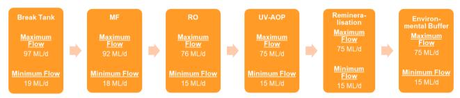
Figure 2 - Flow volumes at each stage of the water recycling process - maximum (75Ml/d) and minimum flow scenarios
