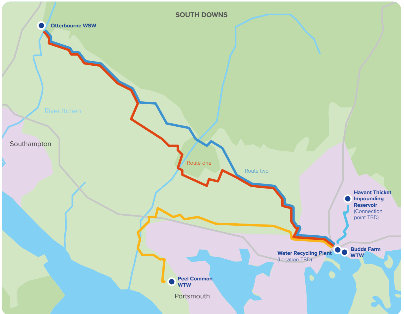
Figure 3: Initial corridor routes between a possible WRP location and Otterbourne WSW
