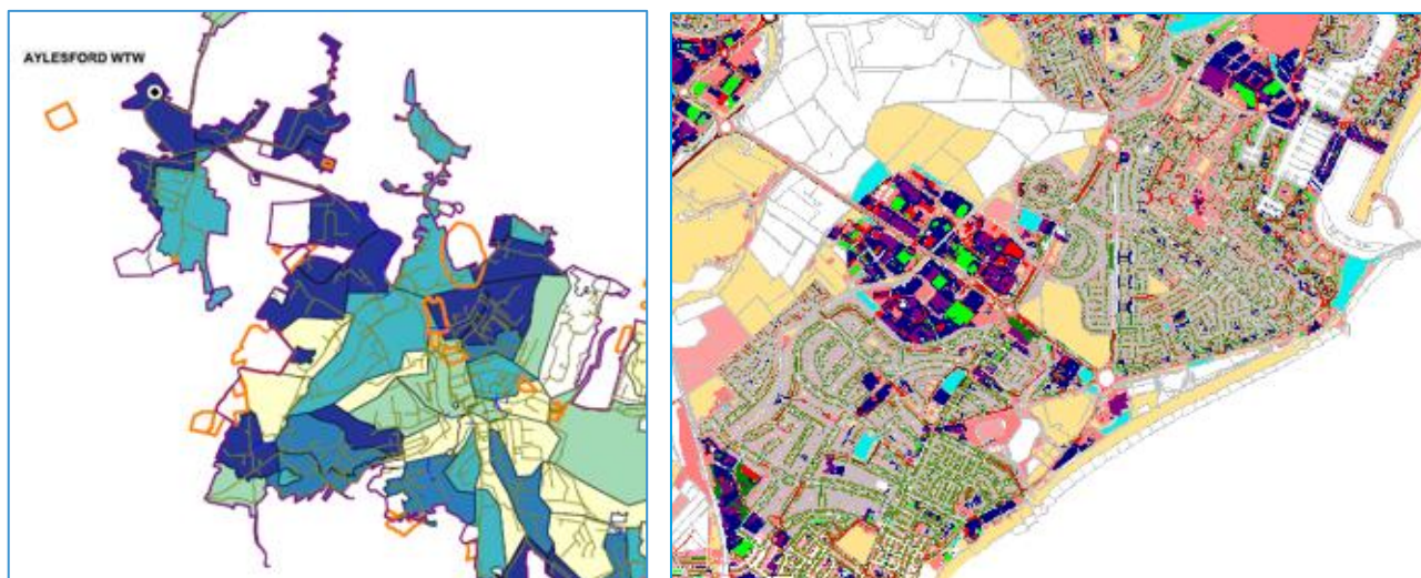
Figure 8: Example visualisations showing a sub-catchment sewer capacity assessment (left), and sources of rainfall run-off and sinks to identify potential opportunities for SuDS (right)
