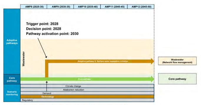
Figure 7: Wastewater: Adaptivity pathway 2 – Surface water separation initiative
